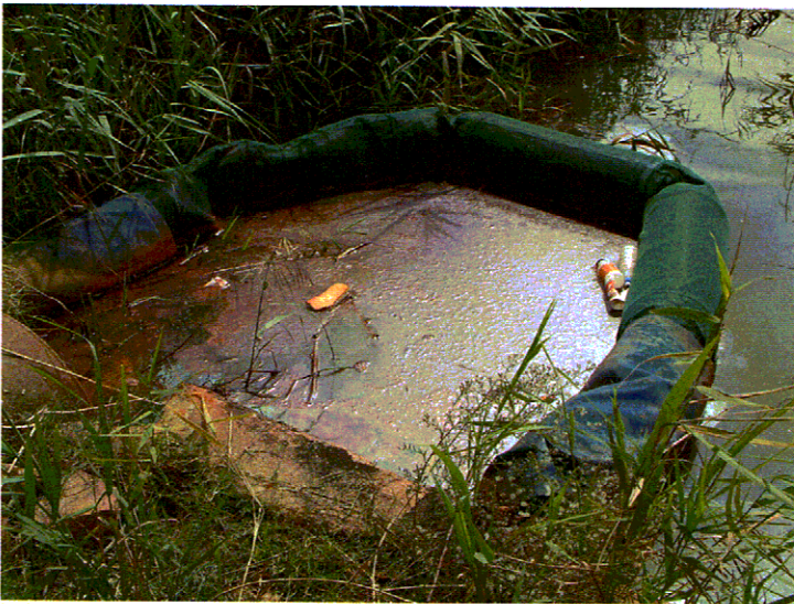
The litter boom in operation at S8
